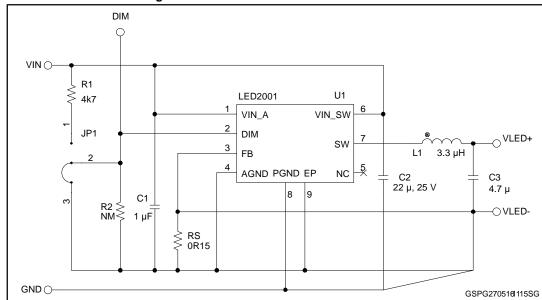
Figure 1: STEVAL-ILL054V2 circuit schematic
