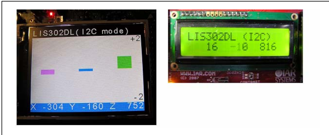
Figure 20. STM32-MEMS LCD demonstration application running on STM3210B_EVAL (left) and STM3210B_SK_IAR (right)
