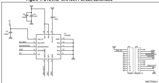
Figure 1. STEVAL- MKI136V1 circuit schematic
