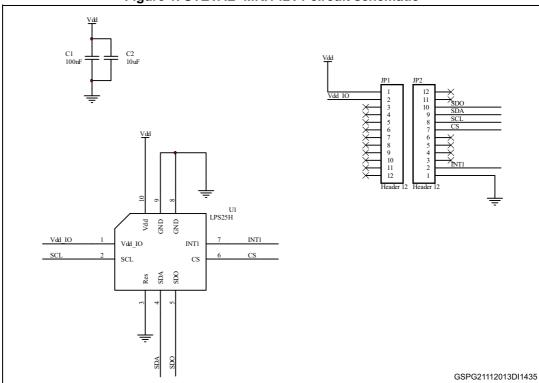
Figure 1. STEVAL- MKI142V1 circuit schematic
