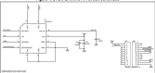
Figure 1. STEVAL-MKI151V1 circuit schematic
