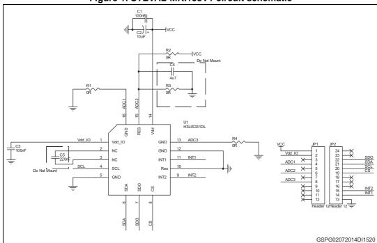
Figure 1. STEVAL-MKI153V1 circuit schematic
