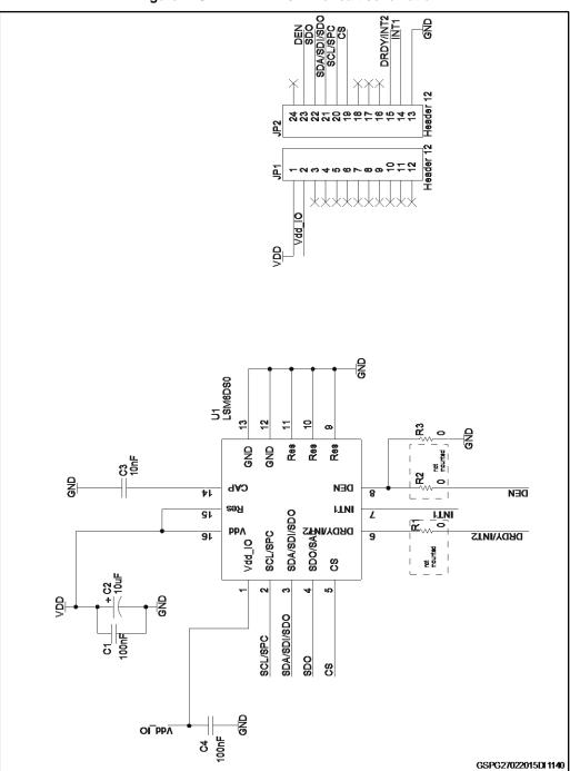
Figure 1: STEVAL-MKI161V1 circuit schematic
