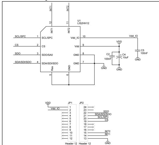
Figure 1: STEVAL-MKI164V1 circuit schematic
