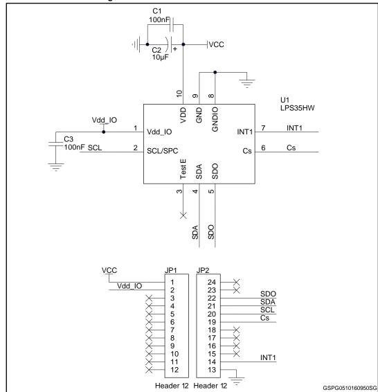
Figure 1: STEVAL-MKI177V1 circuit schematic
