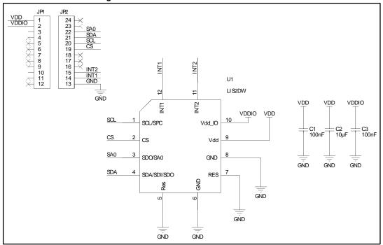
Figure 1: STEVAL-MKI179V1 circuit schematic
