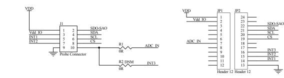
Figure 2. STEVAL-MKI200V1 board schematic
