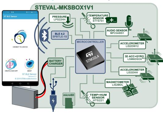
Figure 1. SensorTile.box block diagram
