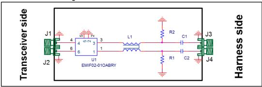
The board schematic shows four RF SMA connectors (J1, J2, J3 and J4) for the following connections:
