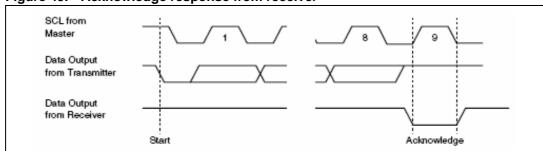
Figure 50. Bus timing requirements sequence
