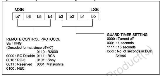
When b7 = '0', incoming RC data is output on SDA in **decoded format** where the Device Address, Start Bit, Toggle Bit and Data Bits are sent. Note that the default location is 0x00 for the first device address. This order of the bits sent is in the same format as the incoming RC data.
