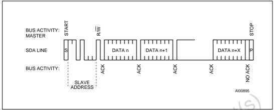
Figure 54. WRITE mode sequence
