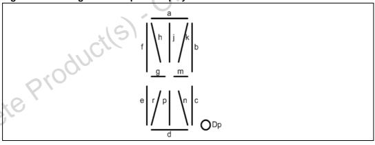
For a display with segment configuration as in *Figure 16*, the location of "a" segment represented by bits b3-b0 corresponds to "0000". Location of b segment corresponds to "0001". Location of c segment corresponds to "0010" and so on.
