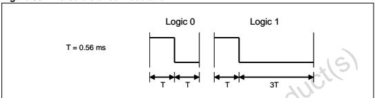
Figure 31. The transmitted waveform for NEC protocol
