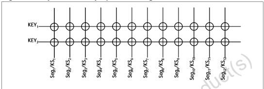
The data of each key is stored as illustrated below and is read by a read command, starting from the most significant bit.
