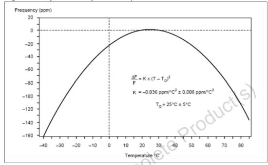
Figure 12. Crystal accuracy across temperature
