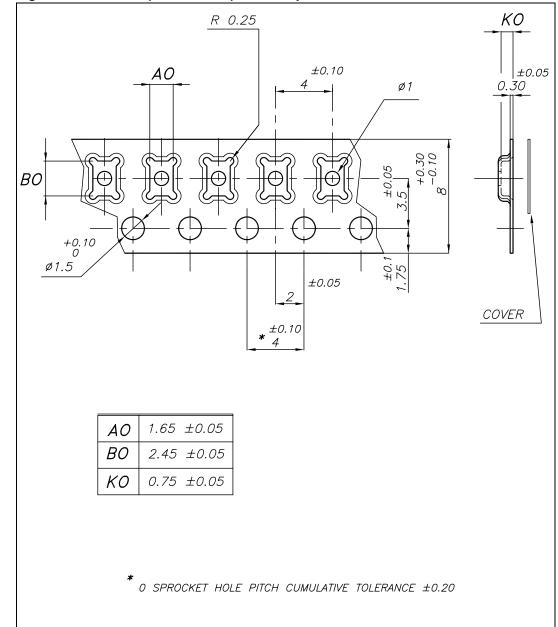
Figure 8. QFN12L (2.2 x 1.4 mm) carrier tape information
