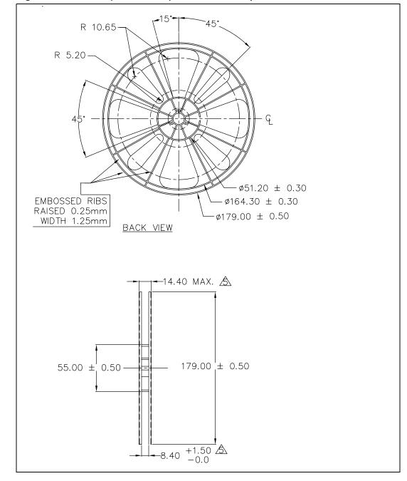
Figure 6. QFN12L (2.2 x 1.4 mm) reel for carrier tape information
