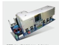
STEVAL-ISW001V1: 2.5 kW double switch forward, 130 A arc welding MMA demonstration board based on the STGW35HF60WD
