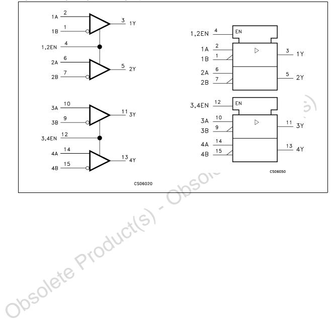
Figure 2. Logic diagram and logic symbol
