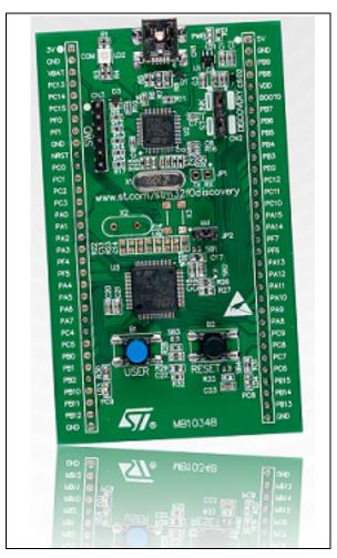
Based on the STM32F051R8T6, it includes an ST-LINK/V2 embedded debug tool, LEDs, pushbuttons and an additional prototyping board for easy connection of additional components and modules.
