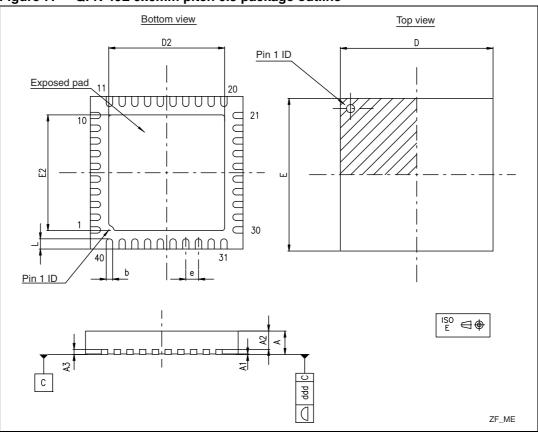
Figure 7. QFN 40L 6x6mm pitch 0.5 package outline
