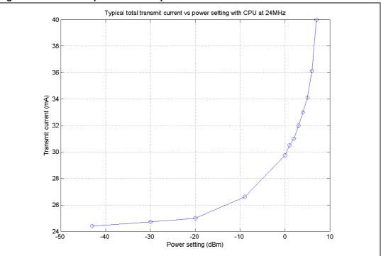
Figure 4. Transmit power consumption
