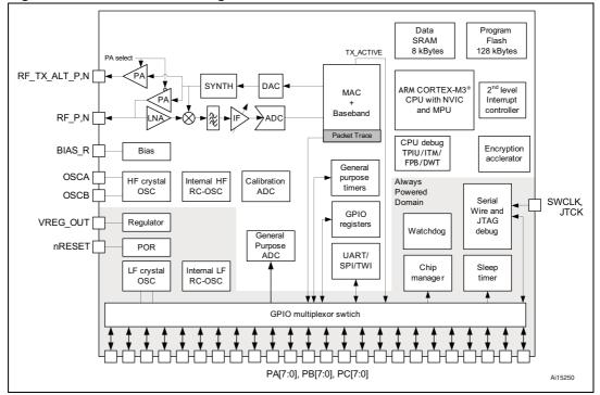
Figure 1. STM32W block diagram
