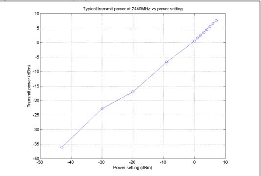
Figure 5. Transmit output power
