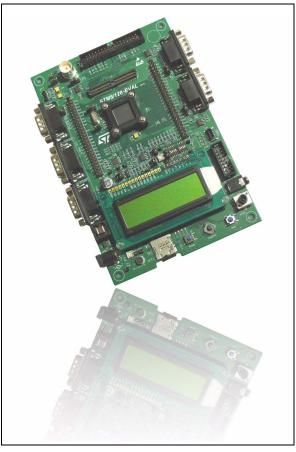
The full range of hardware features helps you to evaluate all peripherals (including motor control, CAN, micro SD Card, smartcard, UART, LIN, IrDA) and develop your own applications. Extension headers make it possible to easily connect a daughterboard or wrapping board for your specific application.
