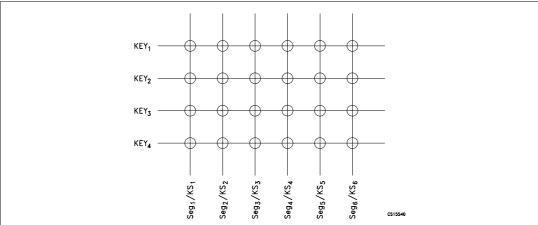
The data of each key are stored as illustrated below, and are read by the appropriate read command, starting from the least significant bit
