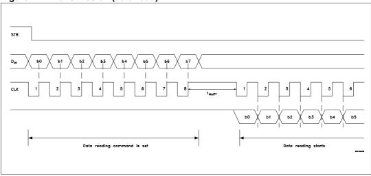
Because the D $_{OUT}$  pin is an N-ch open-drain output pin, be sure to connect an external pull-up resistor to this pin (1 k $\Omega$  to 10 k $\Omega$ ).
