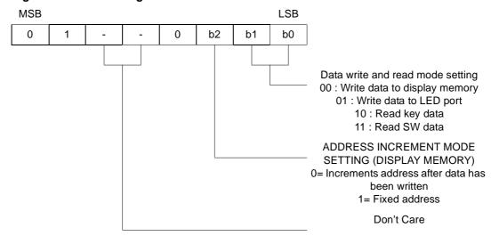
On power application, the normal operation mode and address increment mode are set. Do not use STM86312 in test mode.
