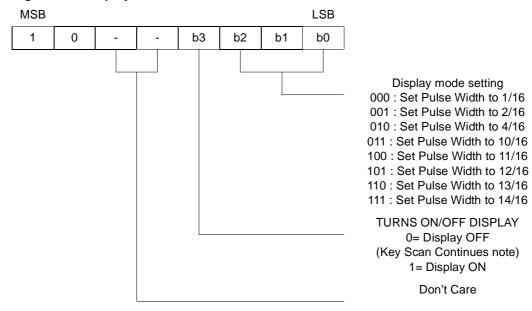
On power application, the 1/16-pulse width is set and the display is turned off.
