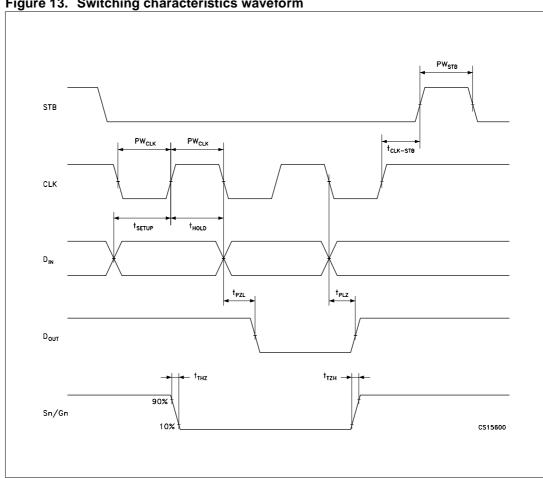
Figure 13. Switching characteristics waveform
