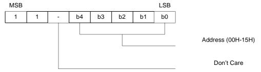
If address 16H or higher is set, the data are ignored, until a correct address is set. On power application, the address is set to 00H.
