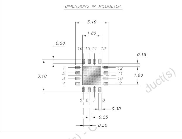
Figure 18. QFN16L footprint - recommended data
