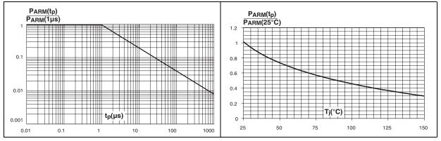
Figure 5. Non repetitive surge peak forward current versus overload duration (maximum values) (TO-220AC)
