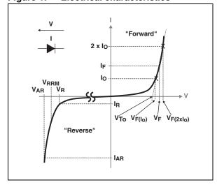
a.  $V_{ARM}$  and  $I_{ARM}$  must respect the reverse safe operating area defined in *Figure 11*.  $V_{AR}$  and  $I_{AR}$  are pulse measurements ( $t_p < 1 \mu s$ ).  $V_R$ ,  $I_R$ ,  $V_{RRM}$  and  $V_F$ , are static characteristics
