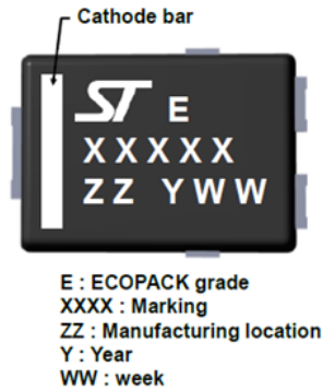
Figure 10. PSMC (TO-277A) marking
