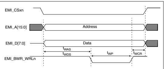
Figure 18. Non-mux write timings
