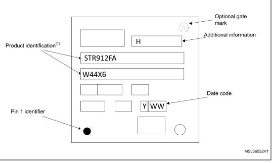
Figure 44. LQFP128 package top view
