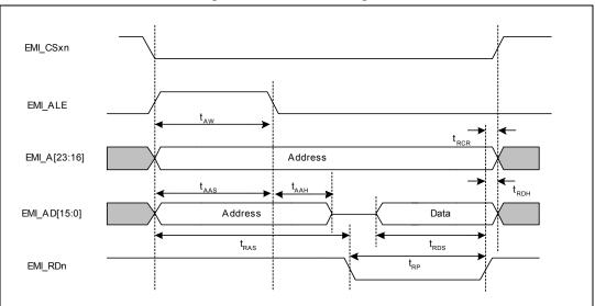
Figure 21. Mux read diagram
