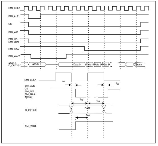
Figure 23. Sync burst write diagram
