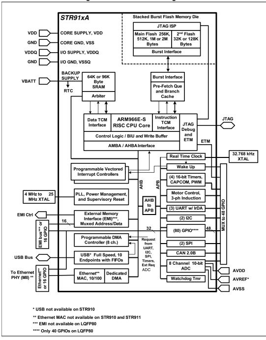
Figure 1. STR91xFA block diagram
