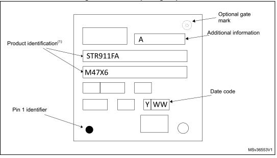
Figure 42. LQFP80 package top view
