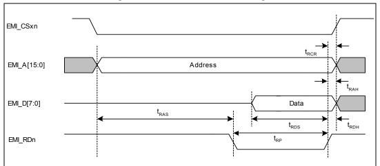
Figure 19. Non-mux bus read timings
