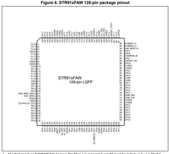
1. NU (Not Used) on STR910FAW devices. Pin 95 is not connected, pin 96 must be pulled up by a 1.5Kohm resistor to VDDQ.
