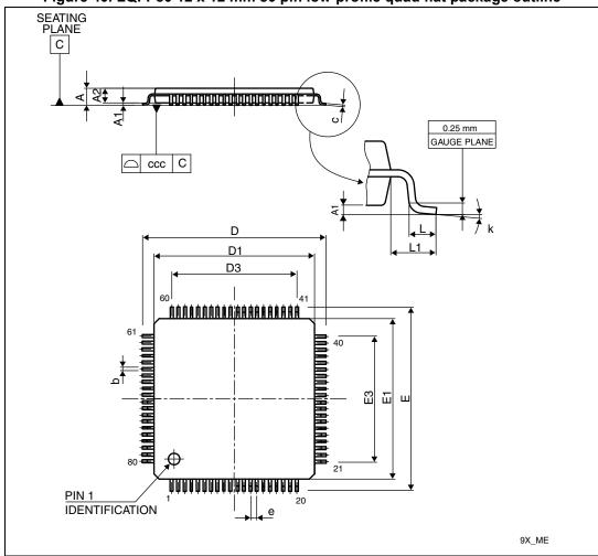
Figure 40. LQFP80 12 x 12 mm 80 pin low-profile quad flat package outline
