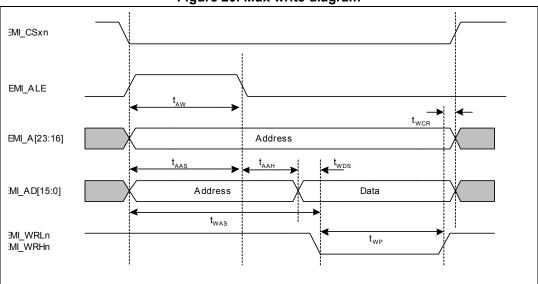
Figure 20. Mux write diagram
