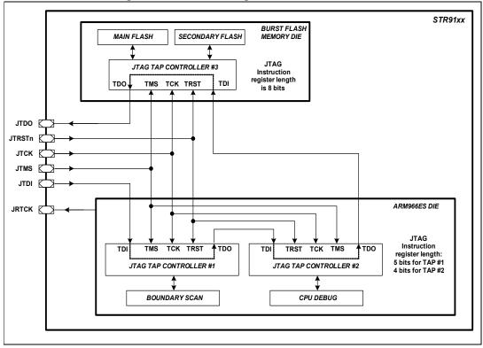
Figure 3. JTAG chaining inside the STR91xFA
