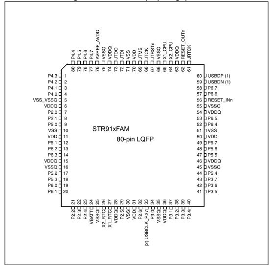
Figure 7. STR91xFAM 80-pin package pinout
