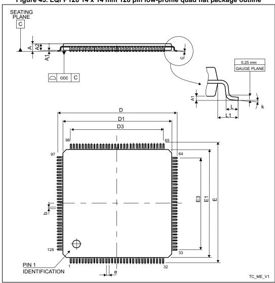
Figure 43. LQFP128 14 x 14 mm 128 pin low-profile quad flat package outline
