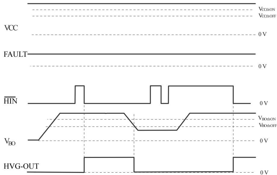
Figure 9. VBO Power-ON and UVLO timing
