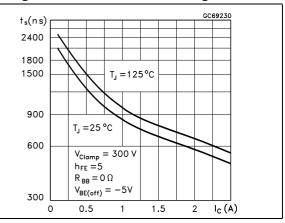
Figure 12. Resistive load fall time
