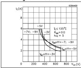
Figure 5. Output characteristics
