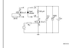
Figure 19: Unclamped inductive load test circuit
