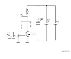
Figure 20: Unclamped inductive waveform
