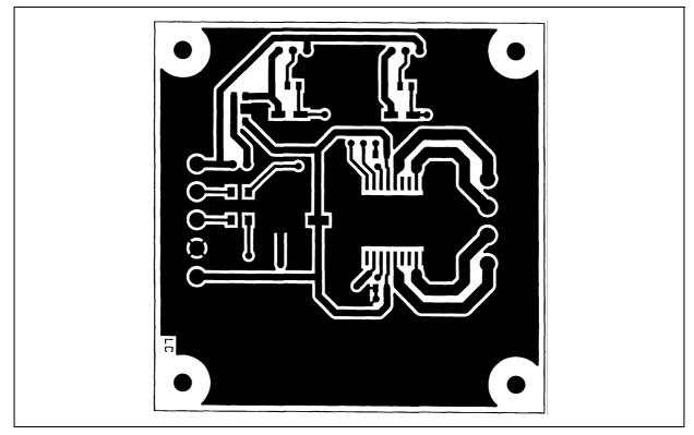
Figure 15. Evaluation Board Top Layer Layout
