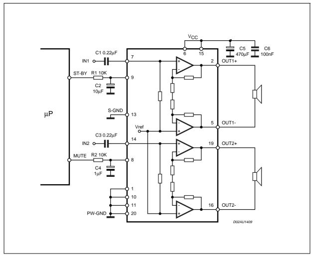
Figure 2. Microprocessor Driving Signals
