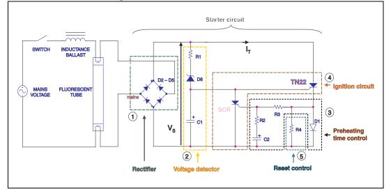
Figure 12. Electronic starter schematic
