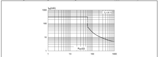
Figure 11. Holding current versus gate-cathode resistance (typical values)
