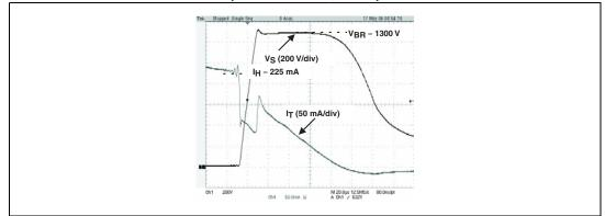
Figure 14. Typical high voltage pulse of an electronic starter circuit (P0130AA SCR, TN22)
