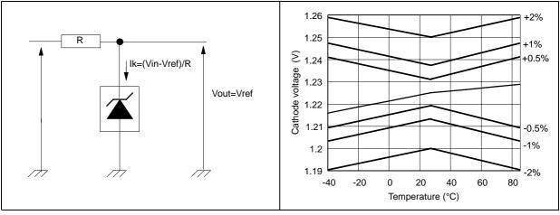
Figure 5. Static impedance versus temperature
