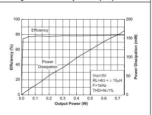
Figure 10. Efficiency vs. output power Figure 11. Efficiency vs. output power 100 150 80 80 05 Dissipation (mW) Power Dissipation (mW) Efficienc Efficiency (%) 09 09 Efficiency (%) -Power 40 Dissipation Vcc=5V Vcc=3V 20 Dissipation RL=8 $\Omega$  +  $\geq$  15 $\mu$ H 20 RL=8 $\Omega$  +  $\geq$  15 $\mu$ H F=1kHz F=1kHz THD+N≤1% THD+N≤1% 0.0 0.2 0.4 0.6 1.0 1.2 0.0 0.1 0.2 0.5 Output Power (W) Output Power (W)
