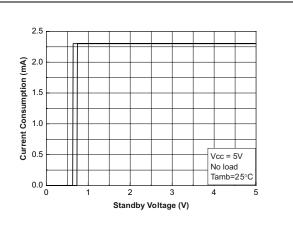
Figure 6. Current consumption vs. standby voltage
