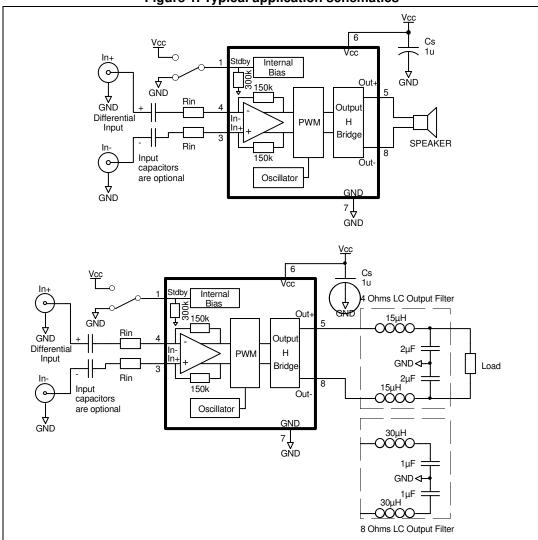
Figure 1. Typical application schematics
