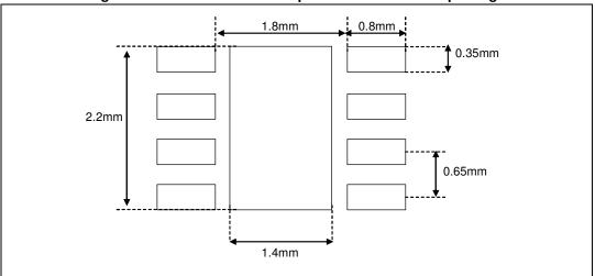
Figure 70. Recommended footprint for TS4962 DFN package
