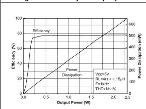
Figure 9. Efficiency vs. output power
