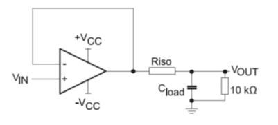
Please note that  $R_{ISO}$  = 33  $\Omega$  is sufficient to make the TSV771 and TSV772 stable whatever the capacitive load.
