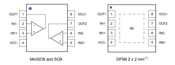
1. The exposed pad of the DFN8 2x2 can be connected to VCC- or left floating.
