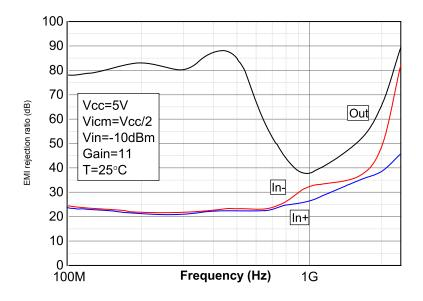
EMIRR performances might be improved by adding small capacitances (in the pF range) on the inputs, power supply and output pins.
