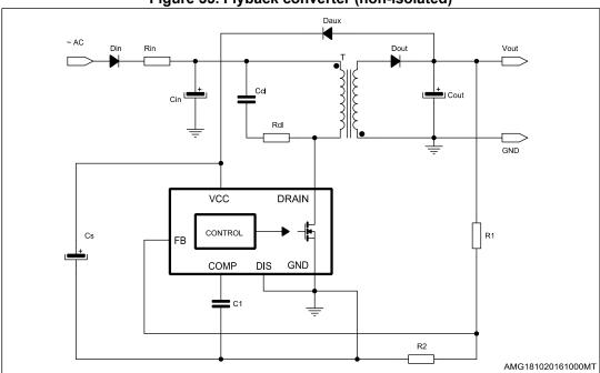
Figure 36. Flyback converter with line OVP (non-isolated)
