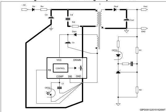
Figure 45. Recommended routing for flyback converter
