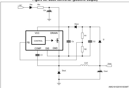
Figure 39. Buck converter (positive output)
