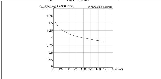
Figure 3.  $R_{thJA}$  / ( $R_{thJA}$  at A = 100 mm<sup>2</sup>)
