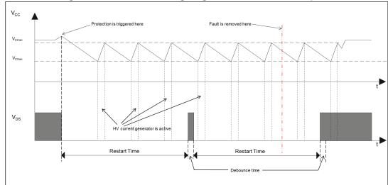
Figure 34. Protection timing diagram with auto-restart option
