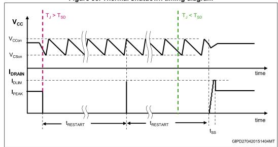
Figure 33. Thermal shutdown timing diagram
