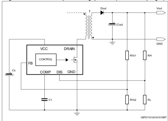
Figure 32. Connection for output overvoltage protection (non-isolated topologies)
