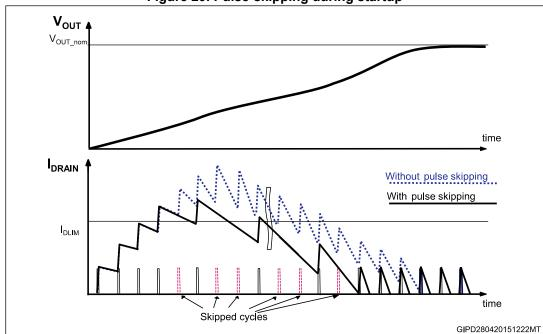
Figure 29. Pulse-skipping during startup
