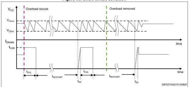
Figure 30. Short-circuit condition
