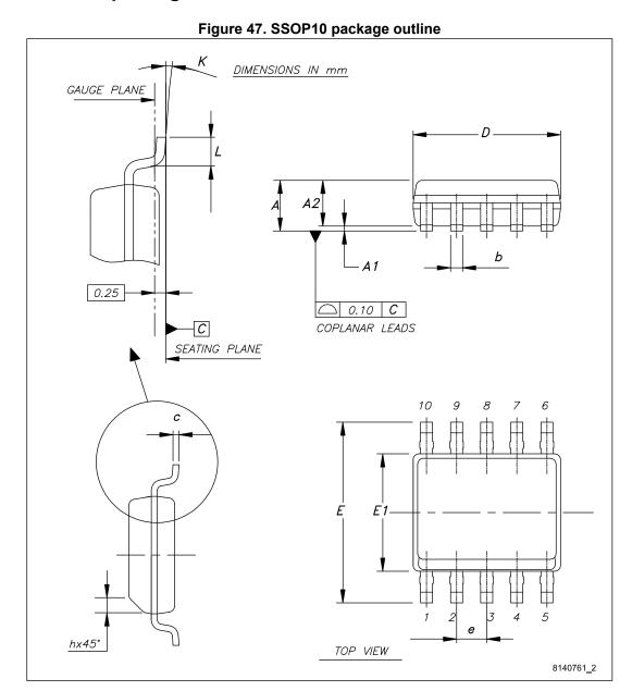
Table 10. SSOP10 package mechanical data
