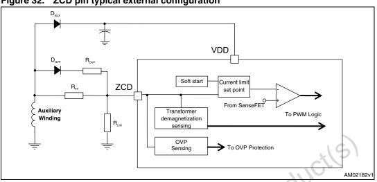
Figure 32. ZCD pin typical external configuration
