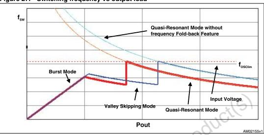
Figure 27. Switching frequency vs output load
