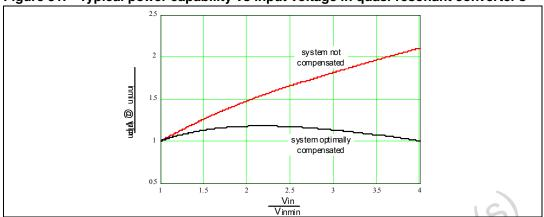
Figure 31. Typical power capability vs input voltage in quasi-resonant converter's
