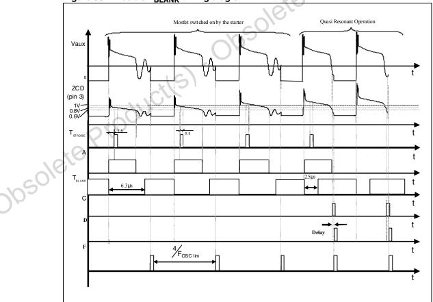
Figure 30. Double T<sub>BLANK</sub> timing diagram
