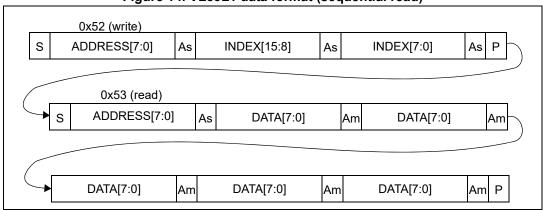
Figure 14. VL53L1 data format (sequential read)
