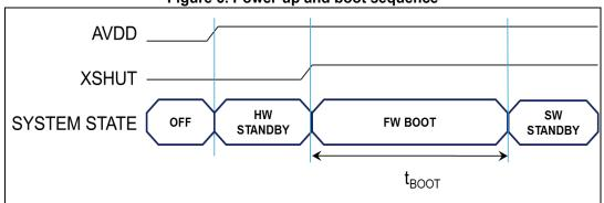
Figure 6. Power-up and boot sequence
