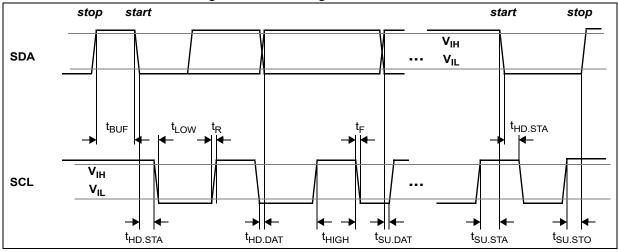
All timings are measured from either  $\rm V_{IL}$  or  $\rm V_{IH}.$
