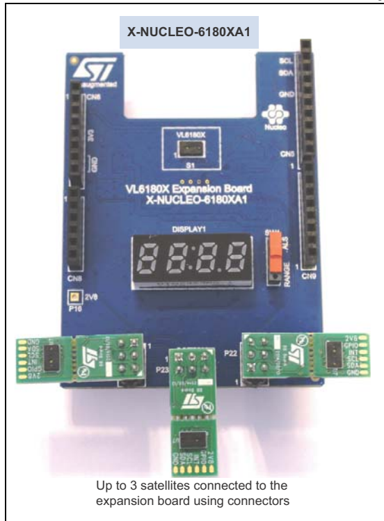
Figure 2. Connection to X-NUCLEO-6180XA1 Nucleo expansion board
