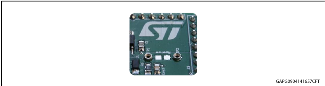
Figure 4: Mounting through-hole sense resistor
