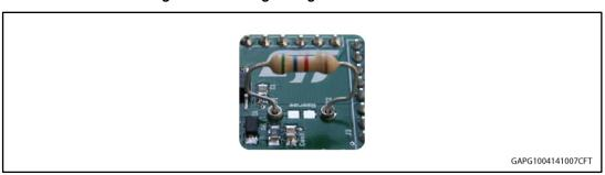
Figure 5: Pads for soldering SMD resistor
