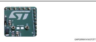
Figure 4: Mounting through-hole sense resistor
