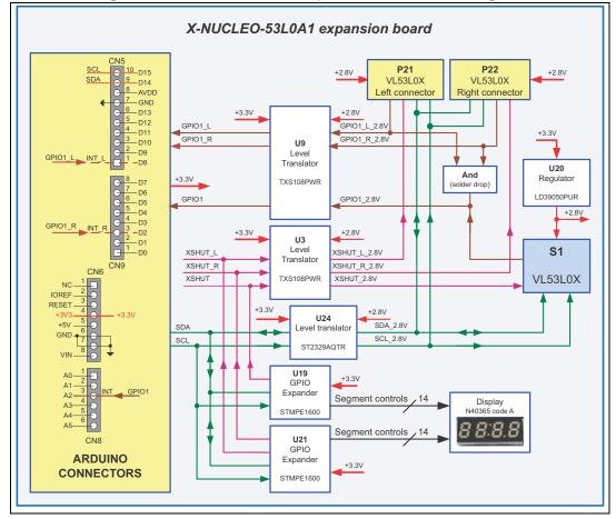
Figure 1. X-NUCLEO-53L0A1 expansion board block diagram
