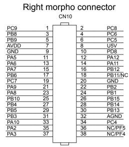
HEADER 19x2 Pass-Through: Female on Bottom and Male on Top
