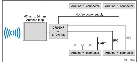
Figure 1. Functional block diagram
