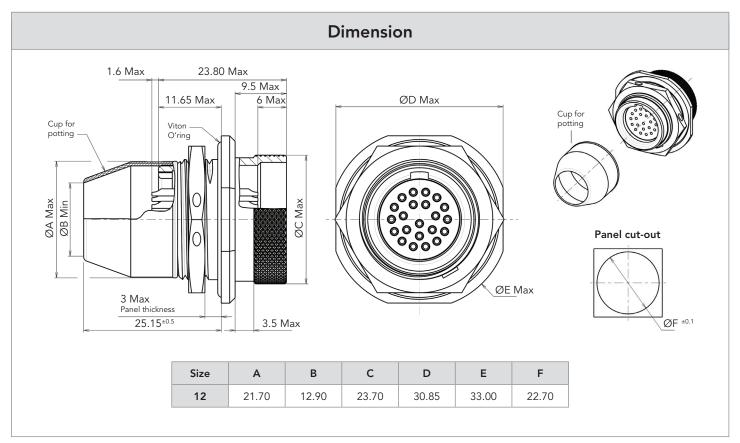
Note: All dimensions are in millimeters (mm)
