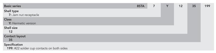
Note: Delivery will contain the cup for potting and the jam nut receptacle not mounted. Consult us for other layouts or shell sizes.
