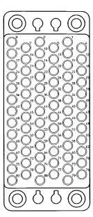
The contact position identification letters or numbers shown in the above diagrams apply to MS-M plug and receptacle connectors. Dimensionally, corresponding types of plug and receptacle mouldings are the same and differ only in that the contact position lettering/numbering of the plug (MS-PM) is a mirror image of that of the receptacle (MS-RM). Note that pins and/or sockets can be used in either the plug or receptacle moulding.
