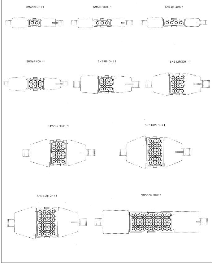
Contact identifications shown are for mating face. Contact identifications of wiring face are identical as shown on the plug arrangements
