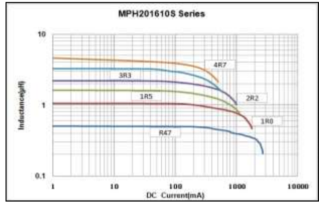
Inductance vs. DC Current Characteristics
