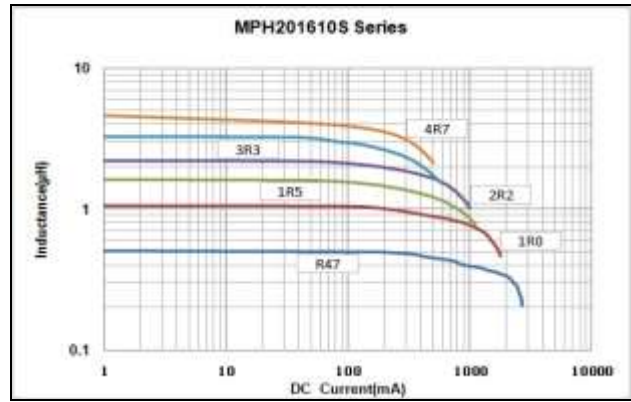
Inductance vs. DC Current Characteristics
