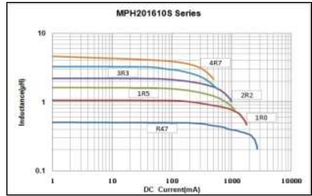
Inductance vs. DC Current Characteristics
