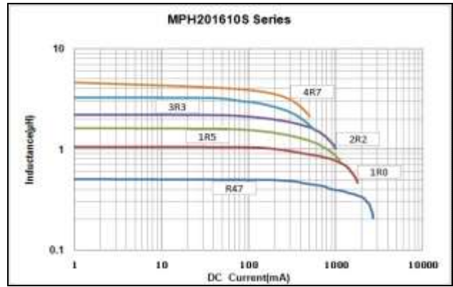
Inductance vs. DC Current Characteristics
